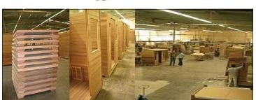
Cedrus Sauna utilizes a heavy duty ten ton press to make sure all the walls are safe, sturdy and built to last a lifetime. Each panel is high pressure sealed for at least five to six hours. After the panels are sealed, they are sent to the double-cut saws where they are
